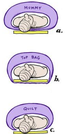
FIGURE 2. Cross-sectional transect showing individual layers of a mummy bag (a), top bag (b), and quilt (c).
