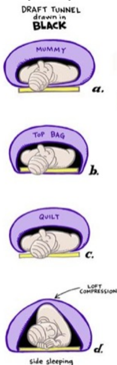
FIGURE 7. Draft tunnels in a mummy (a) vs. top bag (b) vs. quilt (c). Exacerbation of draft tunnels in a top bag while side sleeping (d). The more cross sectional area of the sleep system that is occupied by a draft tunnel (black), the more difficult it is to retain heat in the system.
